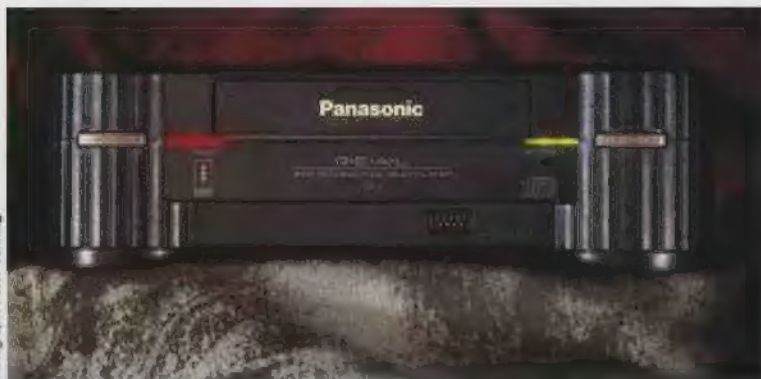
The front of Panasonic's 3DO unit features the CD tray, power button, eject button and joypad port. A red light signifies the machine is on; green means accessing data
